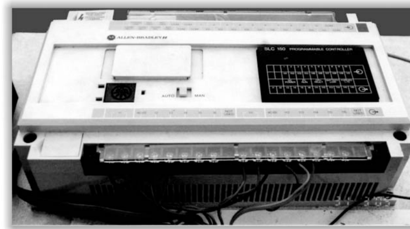
Fig. 12.2 Photographic view of a PLC with fixed input/outputs
